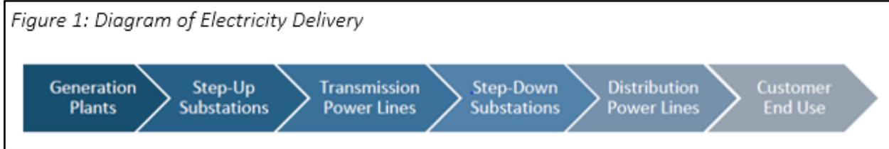
The electrical system consisting of steel towers and/or wood poles and wires in North America are divided into two distinct systems; the high voltage Bulk Electric Transmission System (BETS), and lower voltage distribution systems. Transmission and distribution voltages are divided by the capacity or voltage class as shown in Table 1 below.<sup>8</sup>
